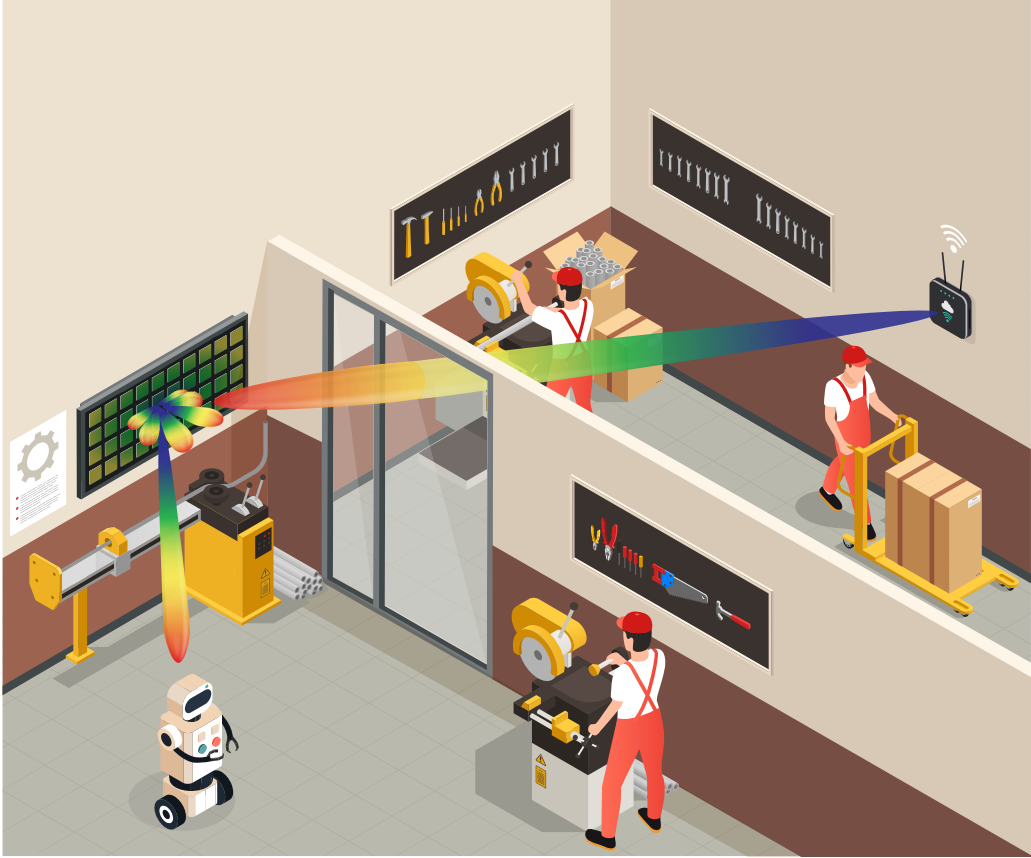
Figure 2.4: Application scenario for an IRS to mitigate blockage in an indoor factory.
